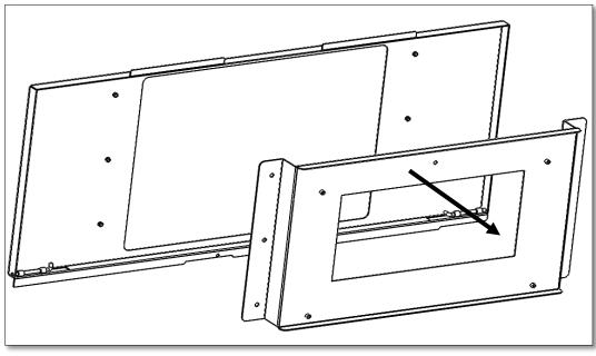
REMOVE MIDDLE PLATE FROM FRONT PANEL BY UNSCREWING 6PCS OF NUT M5
